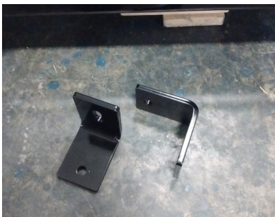
L-bracketes, used for anchoring Tote Enclosure.
